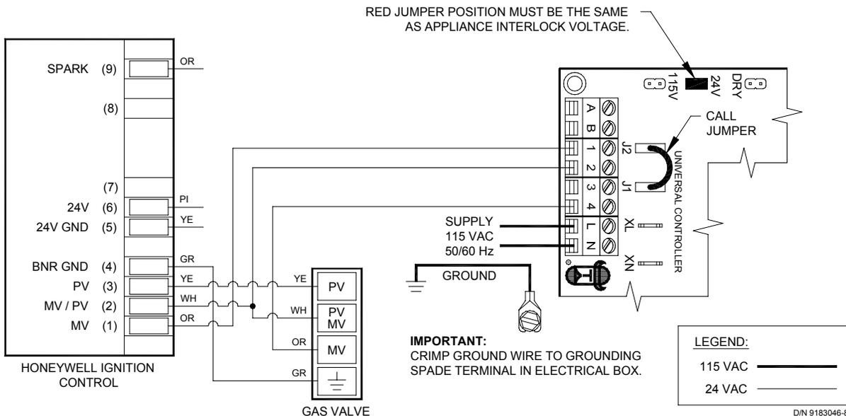
1. Remove the wire on MV at gas valve and connect it on #1 on UC1 terminal block.
