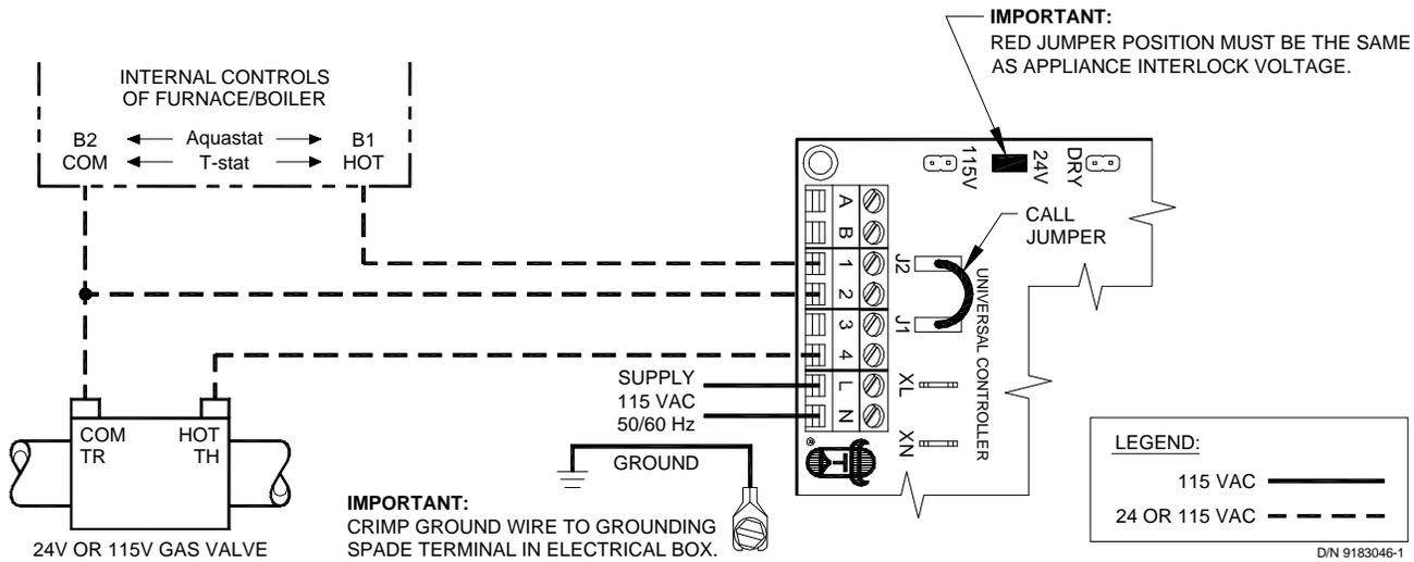
1. Remove the wire on TH or HOT of gas valve and connect it on #1 on UC1 terminal block.
