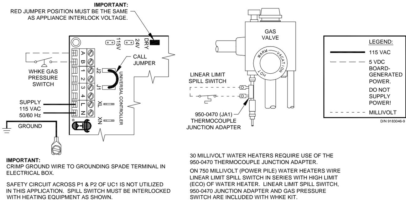
Each millivolt appliance interlocked with the UC1 must have its own WHKE kit installed. The WHKE Gas Pressure Switch actuates the Venter through the A - B Dry contacts. The Linear Limit switch disables the heater in the event of a venting malfunction.
