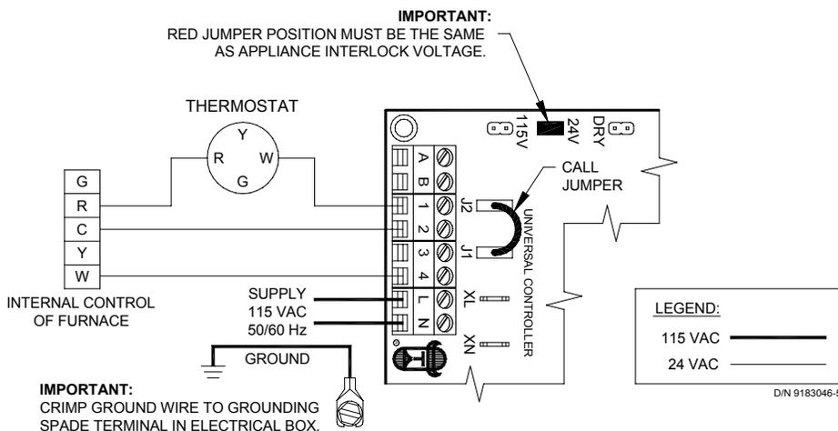
1. Connect W from t-stat to #1 on terminal block of UC1.
