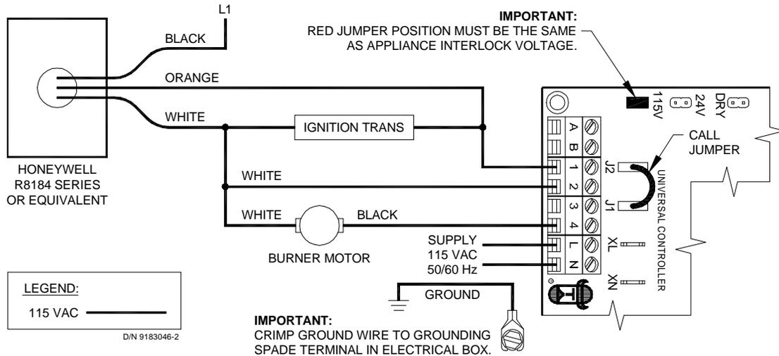
1. Separate the Black burner motor wire from the Orange wire of R8184 Primary Control.
