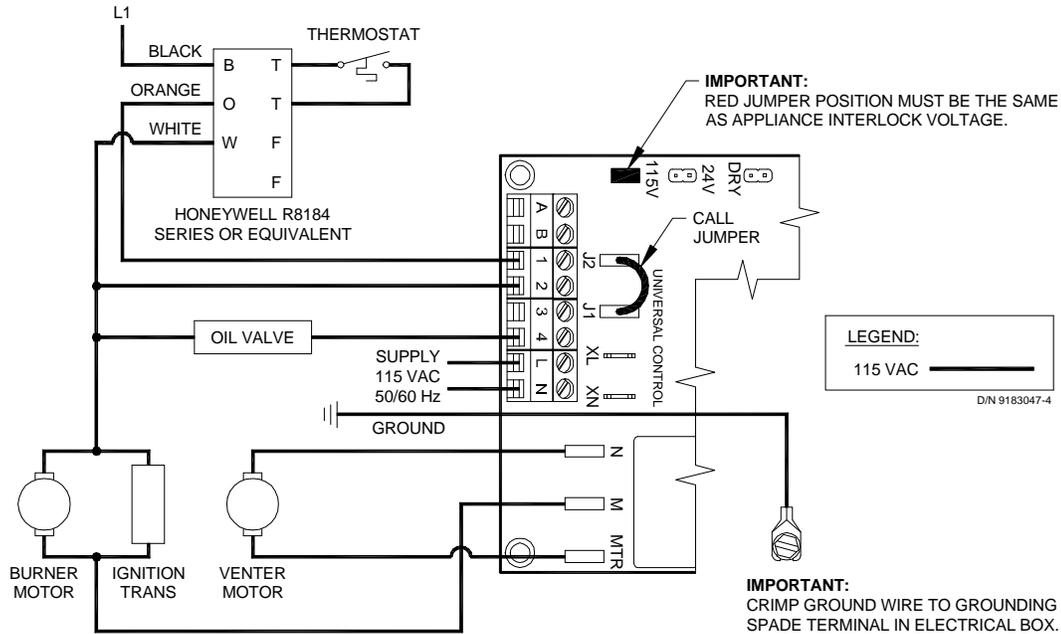
1. Separate the burner motor wire and ignition transformer from the Orange wire of R8184.
