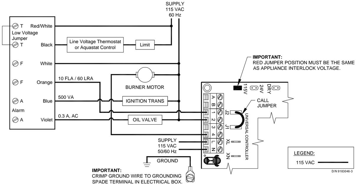
1. Disconnect burner motor wire off the Orange on Carlin.
