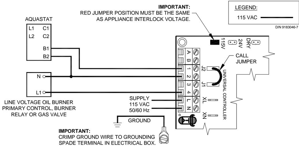
1. Disconnect B1 from L1 of oil burner primary control, burner relay or hot of gas valve and reconnect to #1 on UC1 terminal block.
