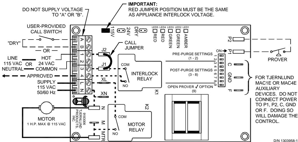
**WARNING:** Disconnect power supply from the UC1 and heating equipment when making wiring connections and servicing the Venter. Failure to do so may result in personal injury and/or equipment damage. LED #5 (RED) should be off with power removed.
