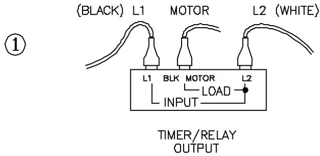
If you are replacing the Timer/Relay of a **VP-2**, **WHK-2** or a **VP-3**, connect the control input voltage as shown in diagram "A".
