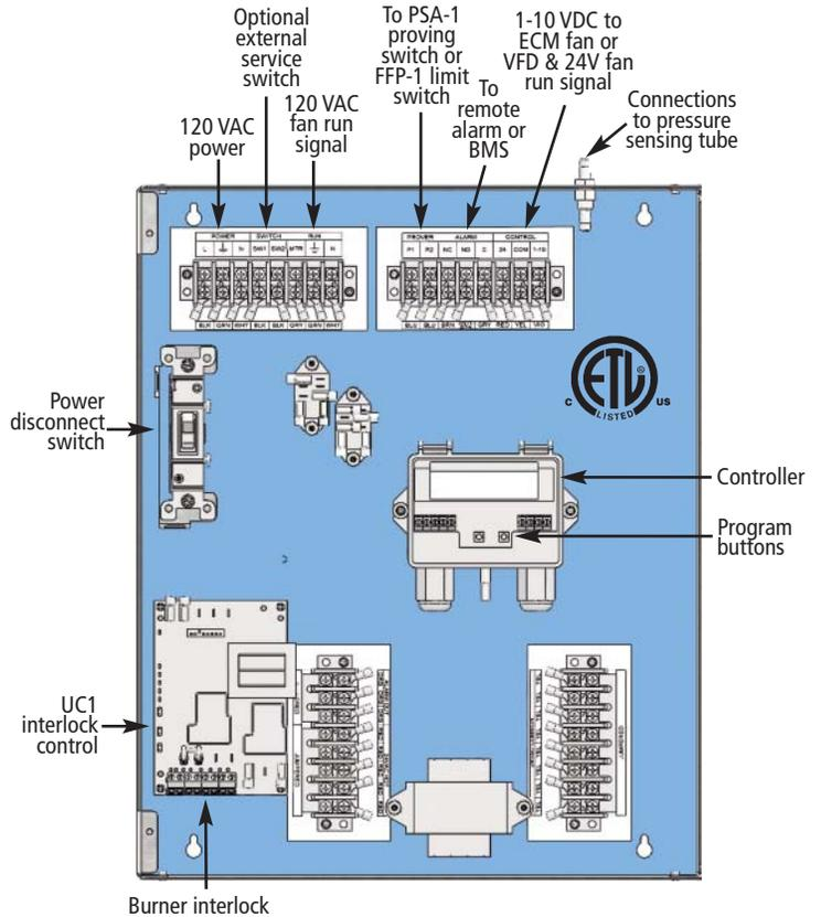
\*Model MPC does not have UC1 interlock. Both controllers include sampling tube and hardware.
