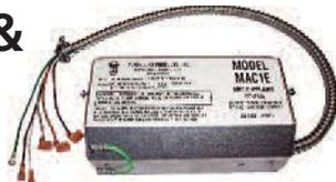
Tjernlund offers MAC controls to interlock additional burner circuits with the UC1 board of MPC1 Controller. Controls are powered by and communicate with UC1 through included color coded whip. Use MAC1E for one additional burner and MAC4E for up to four additional burners.
